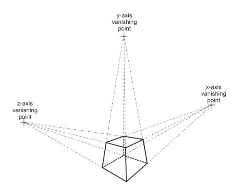
Figure 5-12 Three-Point Perspective of a Cube
