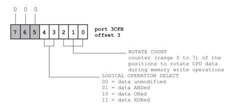
Figure 7-20 Data Rotate Register of the VGA Graphics Controller
