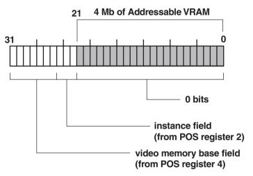
Figure 12-4 Physical Address of Video Memory Bitmap
