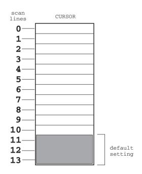
Figure 7-10 Cursor Scan Lines in VGA Systems
