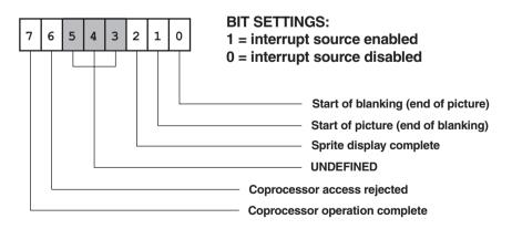
Figure 14-4 XGA Interrupt Enable Register Bitmap
