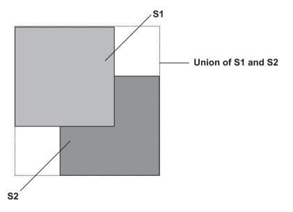
Figure 21-13 Effect of the UnionRect() Function
