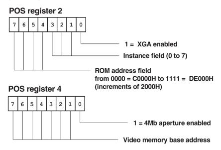
Figure 12-1 XGA Data in POS Registers
