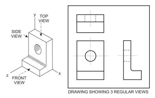
Figure 5-5 Parallel, Orthographic, Multiview Projection
