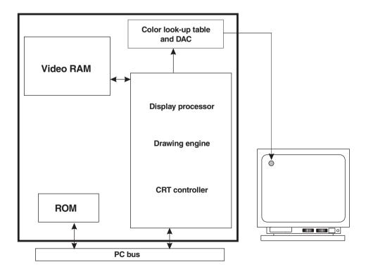
Figure 11-1 8514/A Component Diagram
