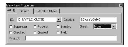
Figure 19-6 Developer Studio Insertion of a Shortcut Key Code
