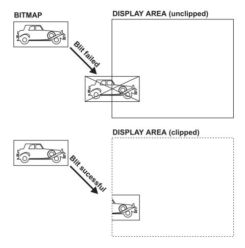
Figure 25-7 Clipping a Bitmap at Display Time
