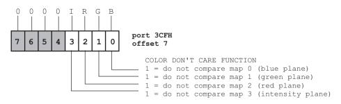
Figure 7-19 Color Don't Care Register of the VGA Graphics Controller
