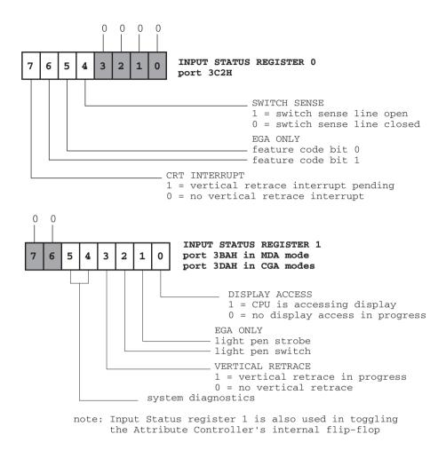
Figure 7-7 VGA Input Status Register
