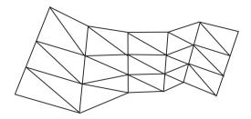
Figure 2-15 Edge Representation of Polygons
