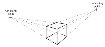
Figure 5-11 Two-Point Perspective of a Cube
