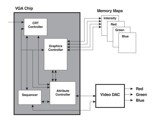
Figure 7-2 VGA System Components
