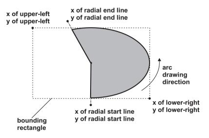
Figure 21-7 Figure Definition in the Arc() Function
