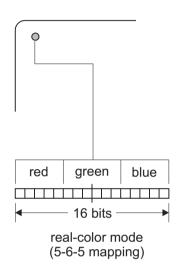
Figure 28-1 Pixel Mapping in Real-Color Modes
