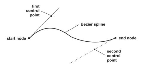
Figure 20-11 Elements of the Cubic Bezier
