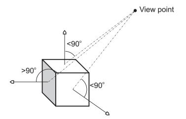
Figure 5-19 Line-of-Sight and Surface Vectors in Culling
