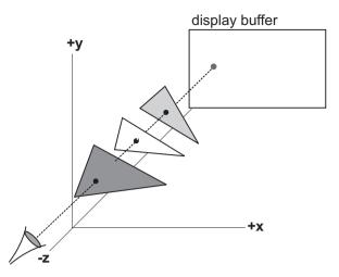
Figure 32-9 Rendering Overlapping Triangles
