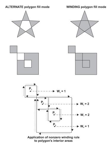
Figure 21-2 Effects of the Polygon Fill Modes
