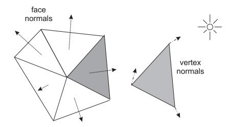
Figure 32-10 Calculating the Vertex Normals
