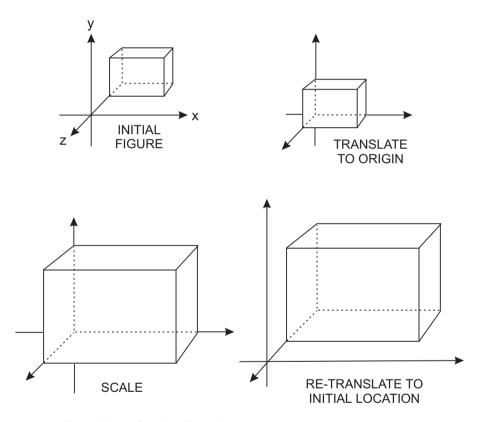
Figure 3-13 Fixed-Point Scaling Transformation
