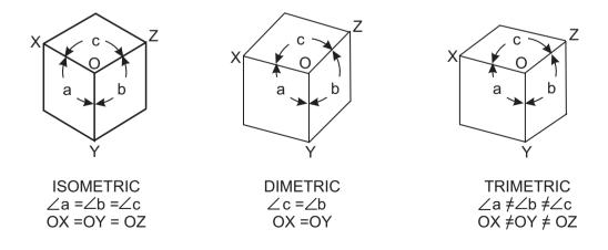
Figure 5-6 Isometric, Dimetric, and Trimetric Projections
