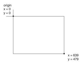
Figure 10-7 Normalization of Coordinates in VGA Mode 18
