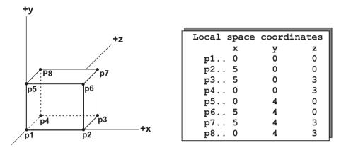
Figure 5-16 Local Space Coordinates of a Cube with Vertex at the Origin
