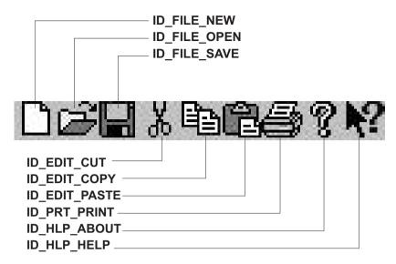
Figure 19-12 "Toolbar.bmp" Button Identification Codes
