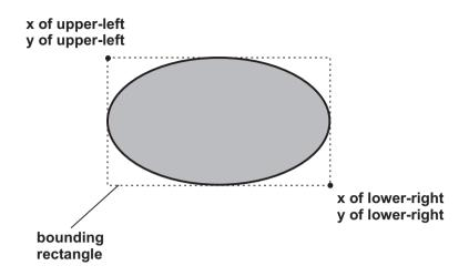
Figure 21-5 Figure Definition in the Ellipse() Function
