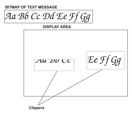
Figure 25-8 Clipper Consisting of Two Rectangular Areas
