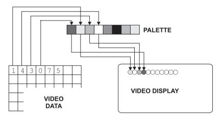
Figure 25-6 Palette-Based Pixel Attribute Mapping
