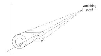
Figure 5-9 One-Point Projection of a Mechanical Component
