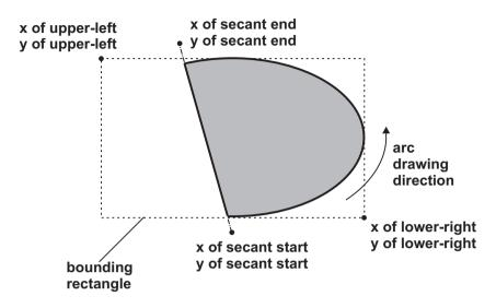
Figure 21-6 Figure Definition in the Chord() Function
