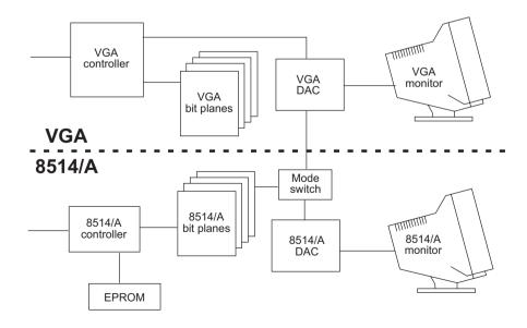
Figure 1-6 Architecture of a VGA/8514A Video System
