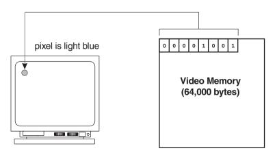
Figure 7-5 Video Memory Mapping in VGA Mode 19
