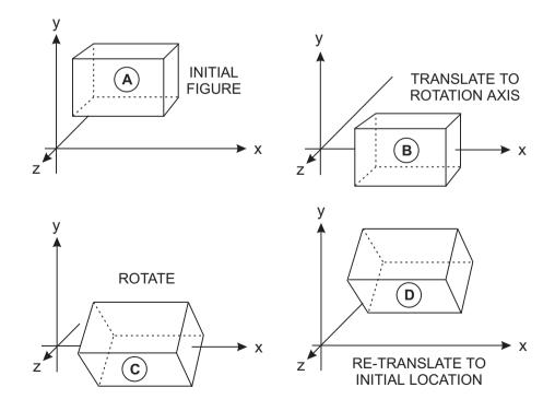
Figure 3-16 Rotation About an Arbitrary Axis
