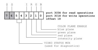
Figure 7-29 Color Plane Enable Register of the VGA Attribute Controller
