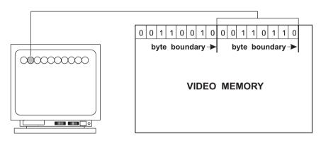
Figure 1-8 Byte-to-Pixel Video Memory Mapping Scheme
