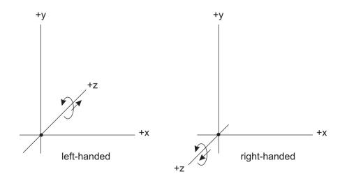
Figure 2-5 Left- and Right-Handed Coordinates
