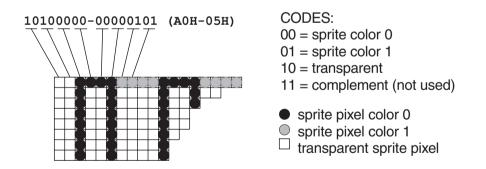
Figure 12-13 Bit-to-Pixel Mapping of Sprite Image
