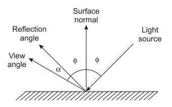
Figure 6-6 Specular Reflection
