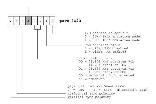
Figure 7-6 VGA/EGA Miscellaneous Output Register
