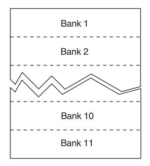
Figure 12-2 Block Structure in XGA 64K Aperture
