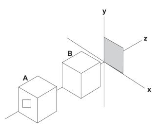
Figure 5-7 Lack of Realism In Isometric Projection
