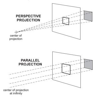
Figure 5-3 Perspective and Parallel Projections
