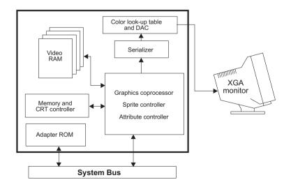
Figure 1-7 XGA Component Diagram
