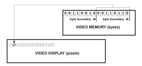
Figure 8-4 Byte-to-Pixel Mapping Example in VGA Mode 19
