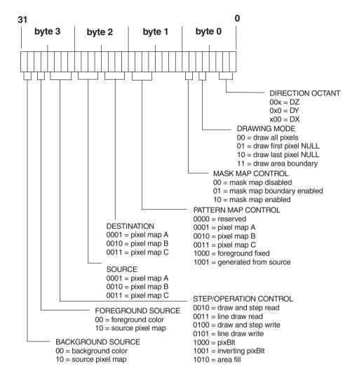
Figure 12-9 Pixel Operations Register Bitmap
