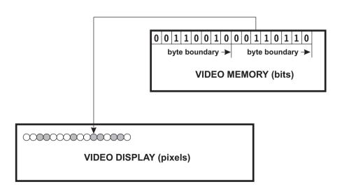
Figure 8-2 Bit-to-Pixel Mapping Example in VGA Mode 18
