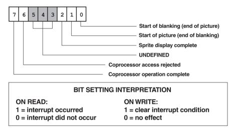
Figure 14-5 XGA Interrupt Status Register Bitmap
