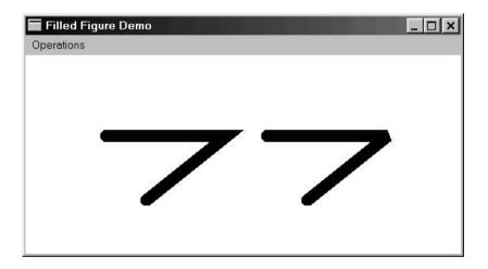
Figure 21-21 Effect of the SetMiterLimit() Function
