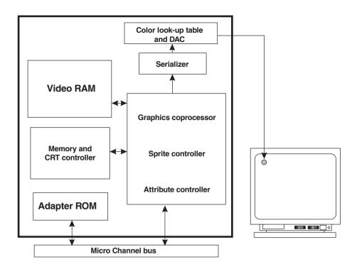
Figure 11-2 XGA Component Diagram
