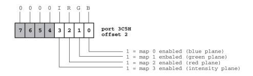
Figure 7-13 Map Mask Register of the VGA Sequencer
