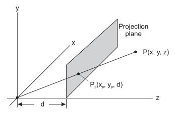
Figure 5-13 Perspective Projection of Point P
