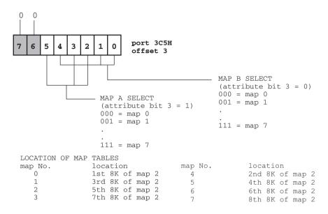
Figure 7-14 Character Map Select Register of the VGA Sequencer
