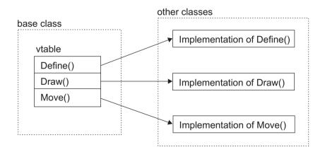
Figure 24-2 The Virtual Function Table (vtable)
