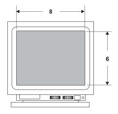
Figure 1-10 CRT with a 4:3 Aspect Ratio
