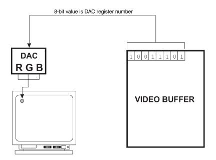
Figure 8-3 Color Mapping in VGA Mode 19
