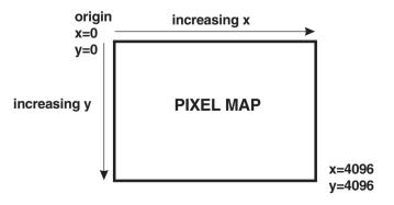
Figure 12-5 Pixel Map Origin and Dimensions
