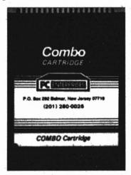
The Combo Cartridge is the most popular PCjr BIOS update cartridge ever sold. The Combo Cartridge Version 3.0 combines all four cartridge routines described above, in a single PCjr cartridge. The Combo Cartridge will speed up the PCjr's memory test, improve and speed up the keyboard and video interfaces, and add all the compatibility updates available for a PCjr. To purchase the Combo Cartridge V3.0, order #18034 (\$89.95).
