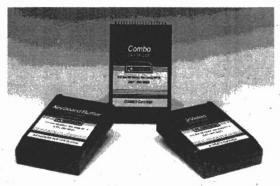
Yes. Three other BIOS update cartridges are available. The Quicksilver Cartridge speeds up the PCjr's memory test that is run each time the computer is turned on. With this cartridge installed, you never have to wait more than a fraction of a second for the PCjr to start loading DOS. More importantly, QuickSilver also corrects a bug that causes double characters, or even no characters, to appear when you use the PCjr's keyboard. To purchase the QuickSilver Cartridge, order #18027 (\$29.95).
