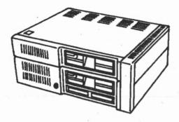
If your PCjr has two disk drives installed, one on top of the other, it is possible that you have a Drive II Enhancement Package made by Rapport, Racore, or Quadram installed. Check the rear of the PCjr for a switch labeled "jr/PC", or a label that describes the add-on option installed on your PCjr. If your PCjr has a Drive II Enhancement package made by one of these companies, you have special memory expansion options.
