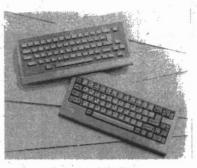
While a wireless interface for a keyboard may sound interesting at first, most PCjr users prefer to have a cable connected to their PCjr. The PCjr keyboard cable allows the keyboard to be used without batteries, and without the keyboard facing the system unit. Keyboard cables also eliminate interference and beeping caused by bright lights and other PCjrs.
