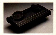
An acoustic modem turns computer signals into audible tones and sends them via a telephone receiver in the modem's cradle.
