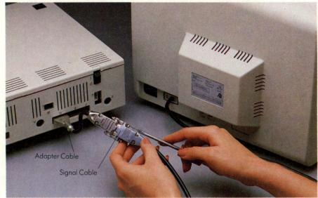
To connect the PCjr to an RGB monitor, turn off and unplug both units, then plug the end of the adapter cable marked D, label up, into the D connector on the back of the system unit. Insert the other end into the free end of the RGB monitor signal cable. Tighten the screws on either side of the connectors. Plug the color monitor's outlet cord into an electrical outlet.
