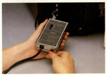
To use the TV set for computer display, set the IBM connector's channel-select switch for channel 4 or channel 3, whichever one is not broadcast in your area, set the switch on the connector's face on COMPUTER, and turn the PCjr on. To return to television viewing, set the switch on the IBM connector's face to TELEVISION.
