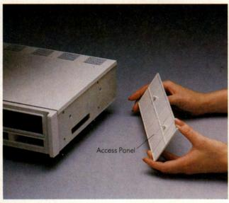
To remove the access panel on the system unit, first turn off the unit and unplug the power cord. Grip the slot at the base of the panel on the right side and pull the panel off. You may need to pry it gently with a nonmagnetized flathead screwdriver.
