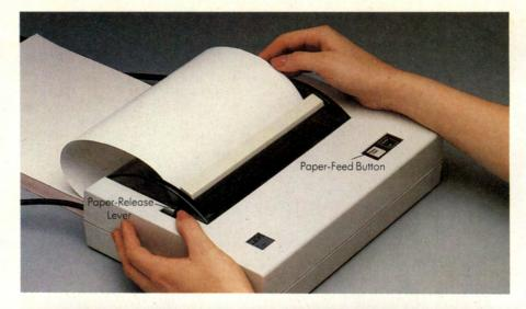
Press and hold down the paper-feed button to advance the paper. Stop when the paper is positioned properly for your first line. To be certain that paper is correctly loaded and the printer is operating, run a printer self-test. Switch off the power and press and hold down the paper feed; switch the power on and when the machine starts printing lines of letters, numbers and symbols, release the feed button. Stop the test by turning off the machine.
