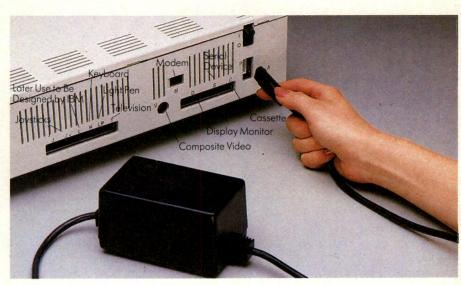
The back of the system unit has 13 input/output slots for cables that link the unit with other parts of the system. The power supply slot, labeled *P*, is at the right side of the back. Before you insert the rectangular plug of the power-supply cable into the system unit, make sure the switch above the connection is in the OFF position. Don't plug the other end of the power-supply cable into an outlet until you have connected the rest of the components to the system unit.
