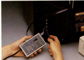
An antenna wire labeled TO TV RECEIVER VHF TERMINAL extends from one end of the IBM Connector for Television. Slip the twin leads of the antenna wire under the television set's VHF screws; use a Phillips screwdriver to tighten the screws (above).
