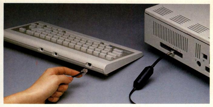
To link the computer keyboard to the system unit with the cable, be sure that the unit's power switch is in the OFF position and unplug the power supply from the outlet bar or wall outlet. Push the cable terminal marked K, with the K facing up, into the connector labeled K on
