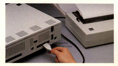
With the power switches of both printer and computer turned off, plug the printer cable into the serial port, which is labeled *S*, at the rear of the computer. Before using the printer, turn on the power first to the computer, then to the printer.
