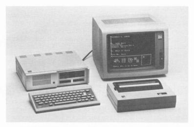
The PCir with keyboard and monitor—a complete system
