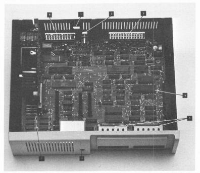
Space for internal modem connector and cable. 2. Connector for composite video. 3. Connectors for (l to r): RF modulator (for TV output), light pen, cable for keyboard, reserved by IBM, 1st joystick, 2nd joystick.
