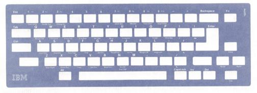
Figure 12-3. An example of a keyboard overlay
