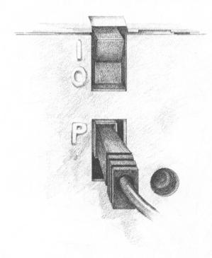
For the transformer, all we have to do is unwrap it, plug one end of the cord into the back of the computer's system unit, and plug the other end into an electrical outlet. Remember, from the last chapter, that the power cord from the transformer plugs into the socket labeled P, as shown in Figure 3-1.
